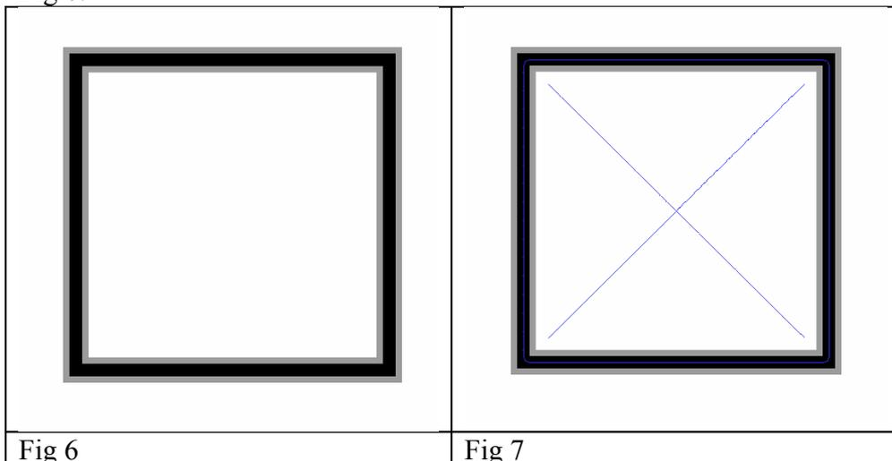
Unfortunately this does lead to a lot of incorrect vectors being created, as in Fig 7, but these can be quickly and easily removed at the end. For sparse maps, with mostly unoccupied space, this technique vastly reduces both the memory and computation requirements of the algorithm.
