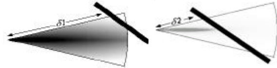
Fig. 2. Sonar beam with an undetected feature at distance \delta l from the emitter. The darker the area, the more strongly it is believed to be unoccupied.
