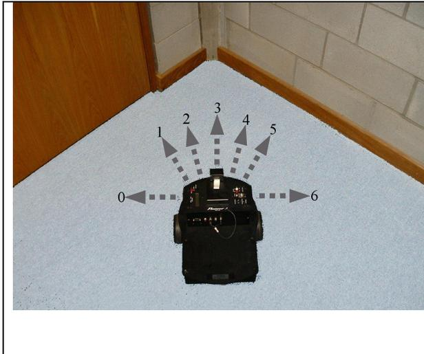
Fig 3.2 (a) Robot facing into a corner often receives incorrect readings from sonars not sufficiently close to  $90^\circ$  from the walls.
